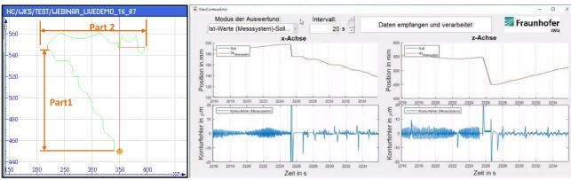
Figure 1: Demo program for the demonstration of the digital twin for path accuracy (left) and graphical user interface depicting the current path accuracy (right)
